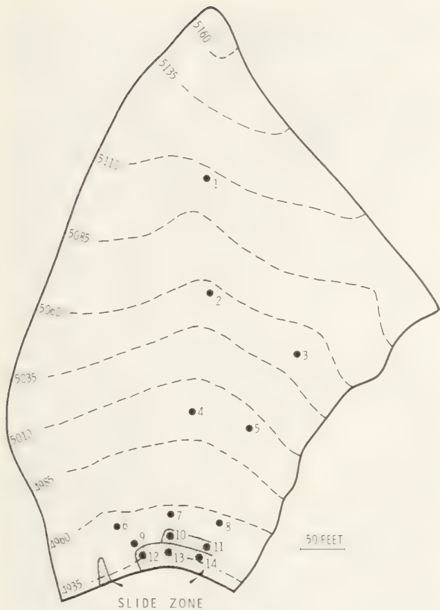
Figure 12. — Location of piezometers and limits of slide zone, Watershed No. 1, Pine Creek study area.
